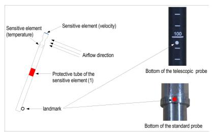
Before any use of the device with an air velocity probe, please lower the protective tube (1) of the sensitive element (except vane probe).
