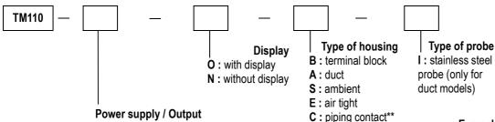
A: Active - 24 Vac/Vdc - 0-10 V P: Passive - 16/30 Vdc - 4-20 mA **Example: TM110-POB**
