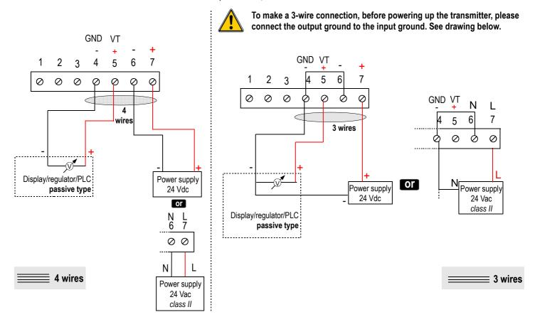
For TM110 - PO and TM110 - PN models with 4-20 mA output - passive :
