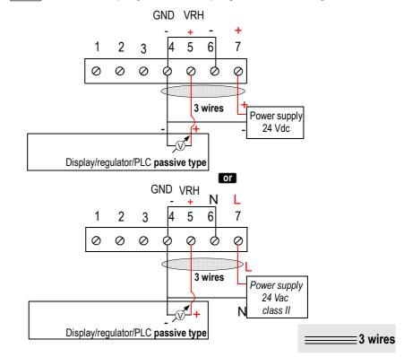
For HM110-PO and HM110-PN models with 4-20 mA output - passive :
