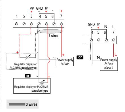
For CP116-PO and CP116-PN models with 4-20 mA output – passive :
